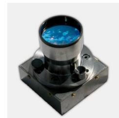
Figure 9-4 MicroASC Star Tracker without Baffle [50]
